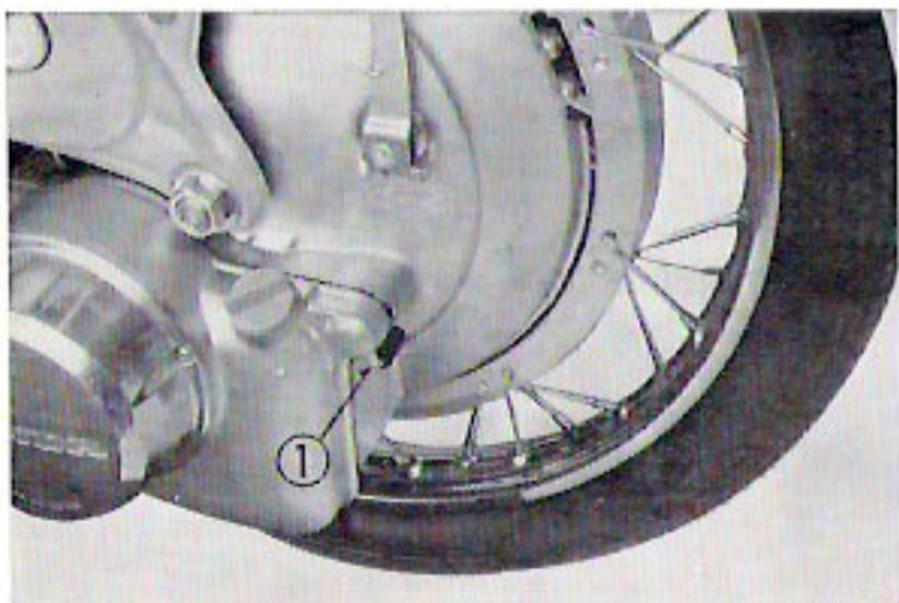
① Clutch disengaging lever
