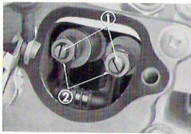
① Adjusting screw ② Lock nut
