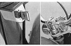
● The handlebar lock which ope● For convenience of the rider, rates with the ignition key is the helmet holder in now atboth simple to use and foolproof. tached on the handlebar.
